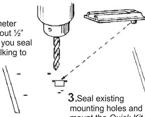
3. Seal existing mounting holes and mount the *Quick Kit* plates over them.
