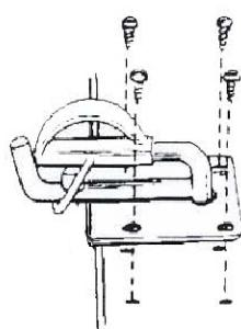
2. Drill a 5/8" diameter (approx.) hole about 1/2" deep. Make sure you seal all holes with caulking to prevent water seepage into the swim platform.
